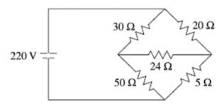
12. When a circuit cannot be simplified by normal series—parallel reduction technique, the stardelta transformation can be used. These two networks will be electrically equivalent if the resistance as measured between any pair of terminals is the same in both star and delta arrangements. Simply the network given in figure using suitable transformations to find an equivalent resistance between A and B.
