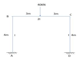
8. Analyze the given beam using **Stiffness Matrix Method** or **Flexibility Matrix method**. Draw the BMD for the beam and Calculate the Maximum positive Bending moment for the span AB and BC. (C.O.No.4) [Application]
