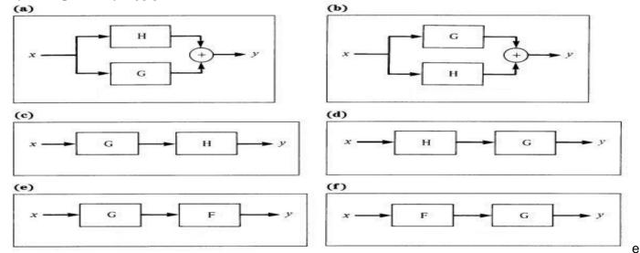
input x[n], determine which of the systems are equivalent.
