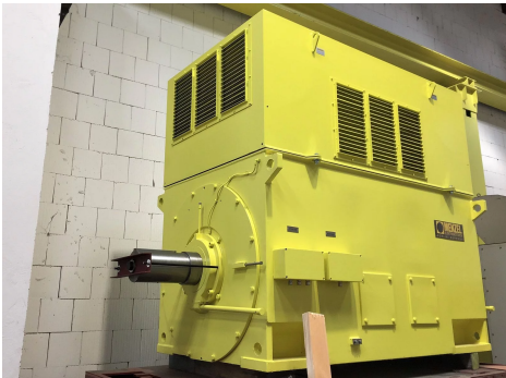
Fig.: MENZEL make Three phase inductor motor for water pumping application in fertilizer plant.
