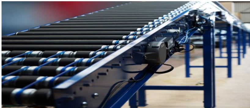
Fig. DC shunt motor in conveyor belt drive
