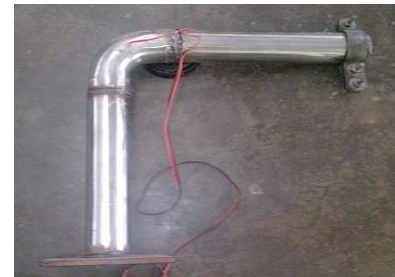
Fig 2: Pipe elbow with strain gauges
