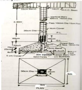
17. For a building at Rameshwaram an estimate has to be prepared for a RCC column shown in Fig.1 with foundation footing. Prepare the estimate for the following items work. A) Earthwork in excavation in foundation, B) Cement concrete 1:4:8 at the base C) RCC work 1:2:4 in footing D) RCC work 1:2:4 in column and E) Steel reinforcing bar.
